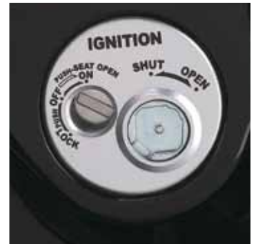
Ignition switch with magnetic security cover
