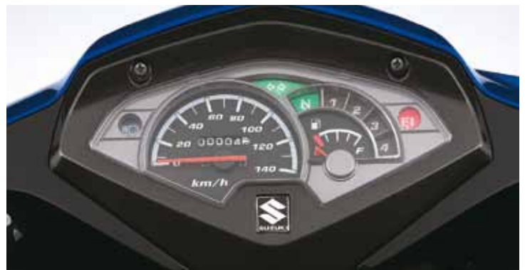
Functional and easy to read instrument panel including a gear indicator
